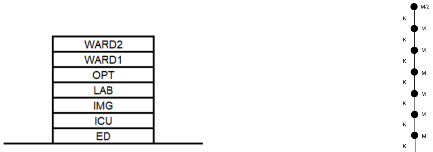
Figure 1 a) A potential medical distribution pattern b) Stiffness and mass distribution of the model
