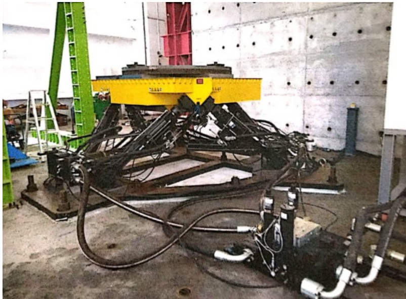
Figure 8. Shaking table system installation (photo courtesy by MTS System Corporation)
