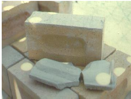
Loss of bond due to overdosing Mortar plasticisers
