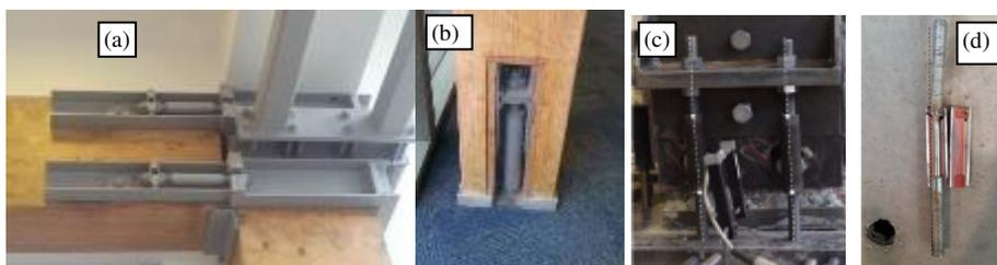
Figure 13. Tests of Externally Mounted Tension-Compression Yielding Devices (MacRae, Gultom and Ma)
