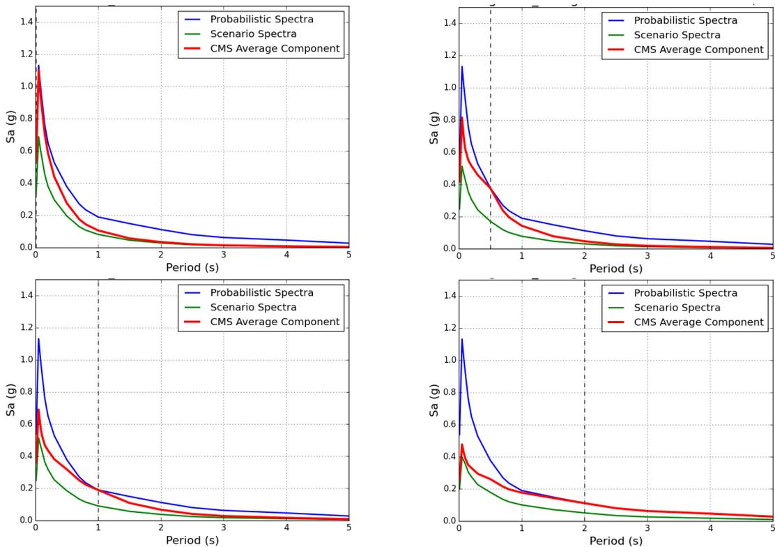
**Figure 2.** Conditional mean spectra (red) for response spectral periods of 0.0 sec (PGA, top left), 0.5 sec (top right), 1.0 sec (bottom left), and 2 sec (bottom right) used to represent the probabilistic UHS spectrum; the dashed vertical lines indicate the CMS periods. The probabilistic (UHS, blue) and median scenario spectra (green) are also plotted for comparison.
