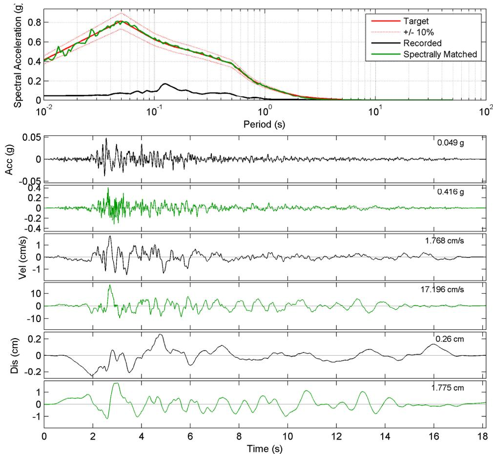
**Figure 3.** Bottom panel: Acceleration, velocity and displacement time histories before (black traces) and after (green traces) the spectral matching process for CMS period 0.5s. Top panel: Response spectrum of the seed time history before (black line) and after (green line) spectral matching to the target spectrum (solid red line).
