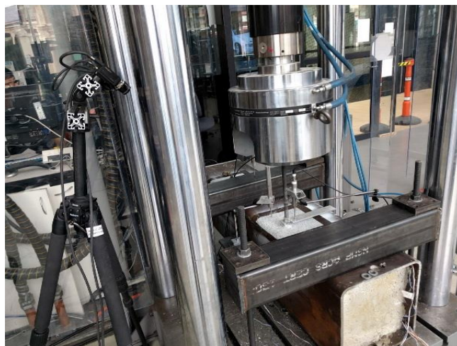
Figure 5: Test setup for pull-out of DHABB from CFSHS 400x400x12.5
