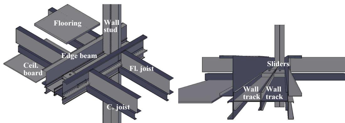
**Fig. 1 Typical modular steel framing with two adjacent slider devices (Jing and Clifton, 2016)**
