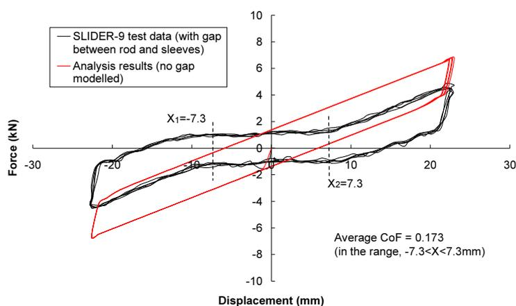
**Fig. 3 Comparative plots of SLIDER-9 and analysis results (1Hz, 6.137kN) (Jing and Clifton, 2016)**
