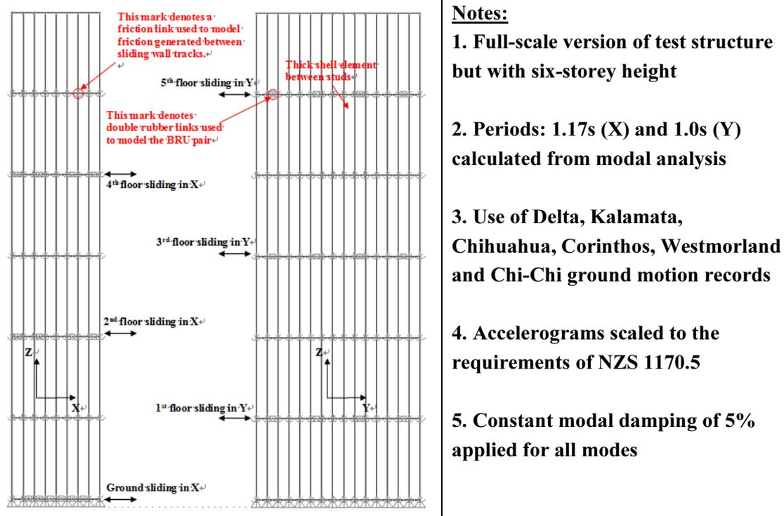
Fig. 6 Six-storey modular steel structure defined in SAP2000 (Jing and Clifton, 2016)
