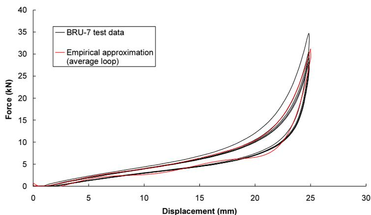
**Fig. 2 Comparative plots of BRU-7 test data and empirical approximation (Jing and Clifton, 2016)**
