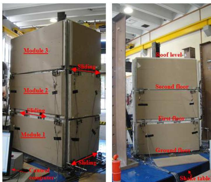
**Fig. 4 Test structure ready to be tested on shake table (Jing and Clifton, 2016)**
