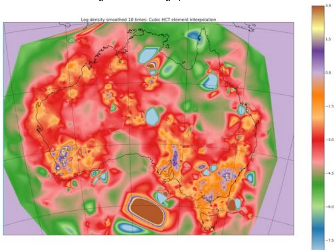
**Figure 9** An interpolation of log-density proxy using Hsieh-Clough-Tocher (HCT) elements applied to natural neighbor smoothed densities. Nine passes of the natural neighbour smoothing have been applied. This produces a C1 continuous function.
