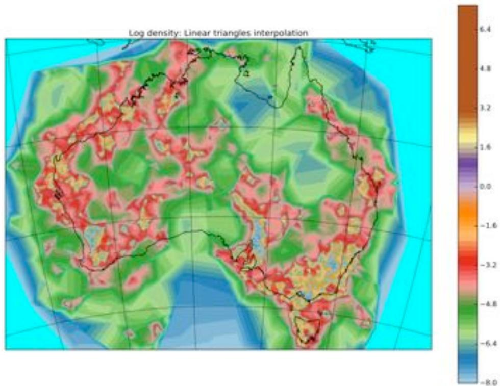
**Figure 6** An interpolation of log-density proxy using a spatially linear interpolation inside each Delaunay triangle.
