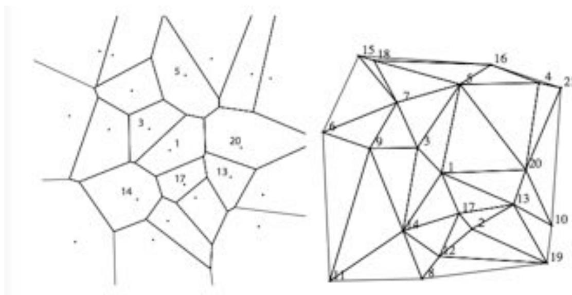
**Figure 2** Voronoi diagram (left) showing nearest neighbour regions about a set of irregular points in the plane. Delaunay triangulation (right) joining nearest neighbour nuclei in the Voronoi diagram. The six numbered cells in the Voronoi diagram share a boarder with cell 1 and are its neighbours.
