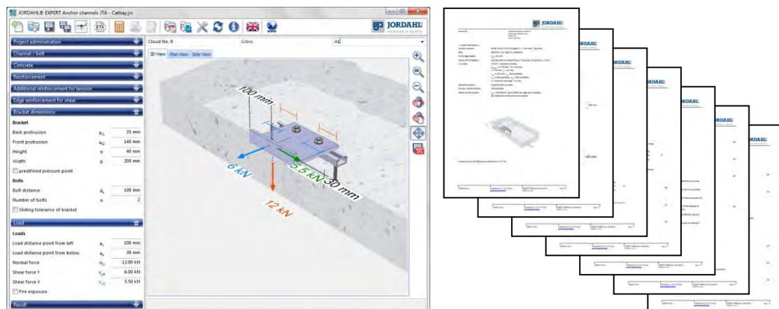
Figure 6. Screenshot of the graphical user interface of a professional anchor channel-channel bolt design software and the print of analysis ready for the checking engineer.
