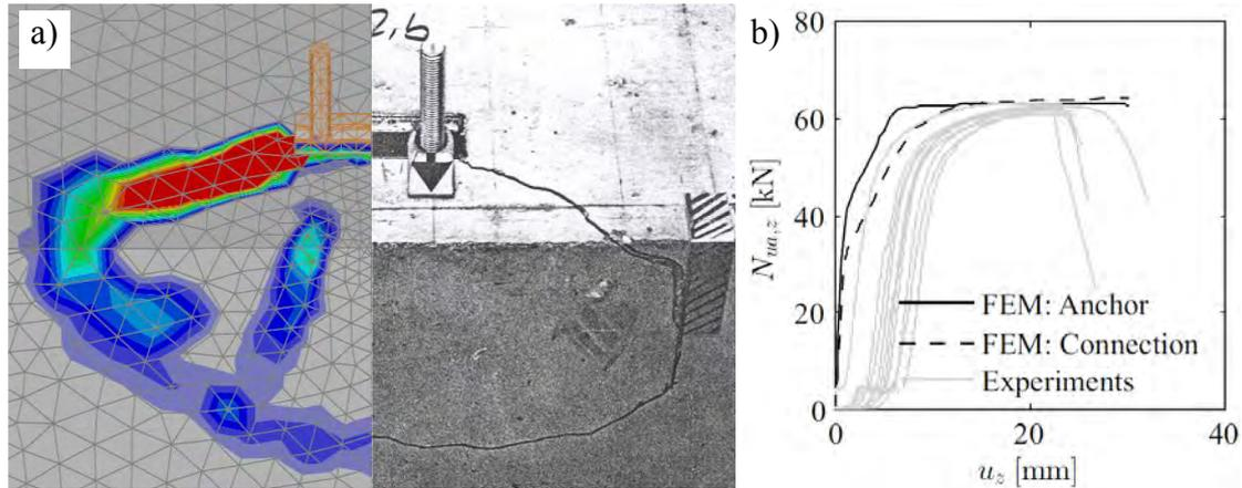
Figure 5. a) Example numerical simulation of experimental test (Potthof (2008)); b) Example load-displacement curves of simulations and tests (Kocur et al. (2016)).
