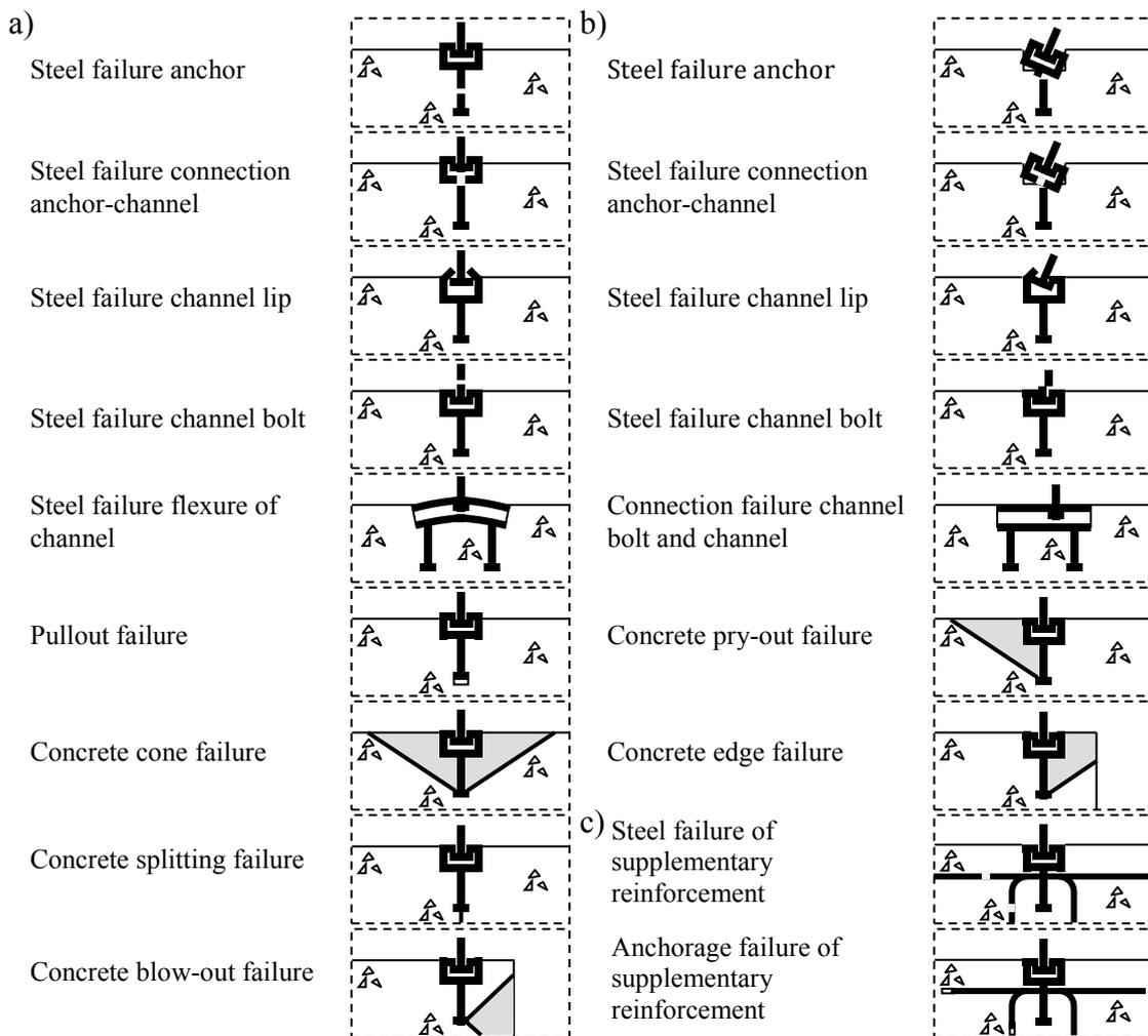
Figure 4. Verifications for anchor channels and channel bolts loaded in a) tension b) shear and c) tension or shear.
