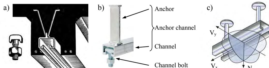
Figure 2. a) Jordahl's invention of anchor channel 1913, b) anchor channel components and channel bolt, c) state-of-the-art systems allow load transfer in all directions.
