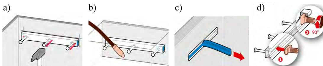
Figure 3. Installation sequence a) attaching of anchor channel to formwork, b) casting of concrete, c) removing of filler, d) twisting-in of channel bolt.
