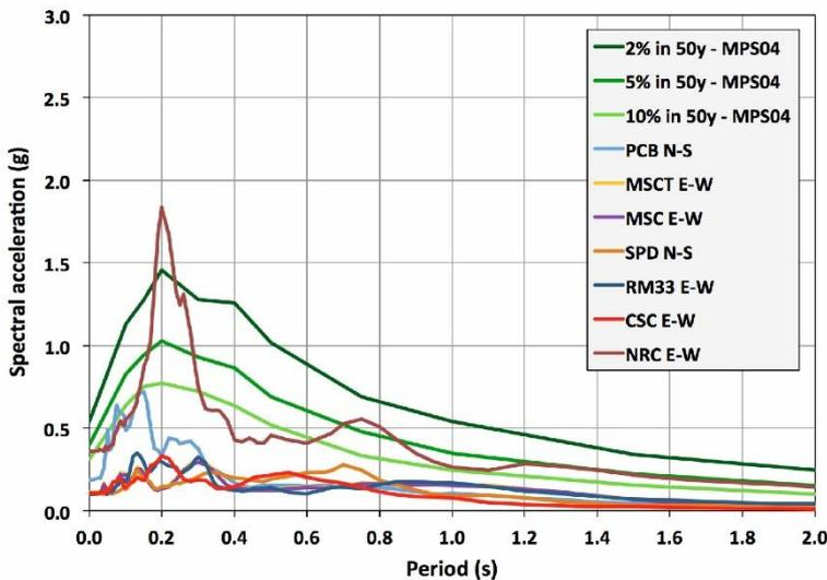
**Figure 7:** Comparison between the maximum horizontal acceleration response spectra (5% damping) of the Amatrice M6.0 mainshock recorded at the stations located between 16 and 25 km from the epicenter and the UHS of MPS04 for soil class B, at a node located at about 20 km to the southeast of AMT, for 2%, 5% and
