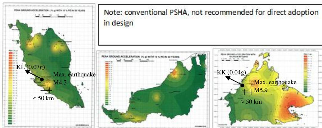
Figure 6: Seismic hazard PGA contours on rock generated by conventional PSHA for the Peninsular, Sarawak and Sabah prepared by local contingent led by Professor Adnan.
