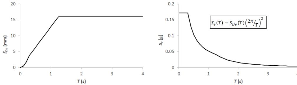
Figure 3 – Response spectrum on rock site for Sarawak and SW Sabah
