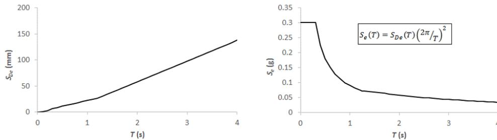
Figure 4 – Response spectrum on rock site for CNE Sabah
