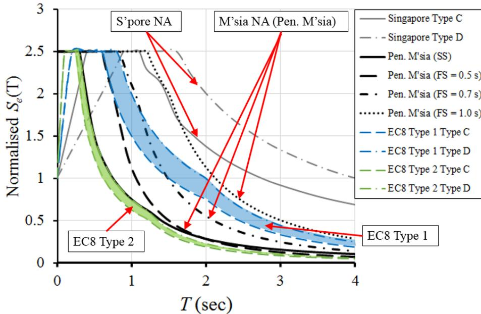
Figure 5 – Normalised spectrum shape comparison of the proposed response spectrum model in the Malaysia NA (Peninsular Malaysia) with the generic EC8 for Europe and the Singapore NA.
