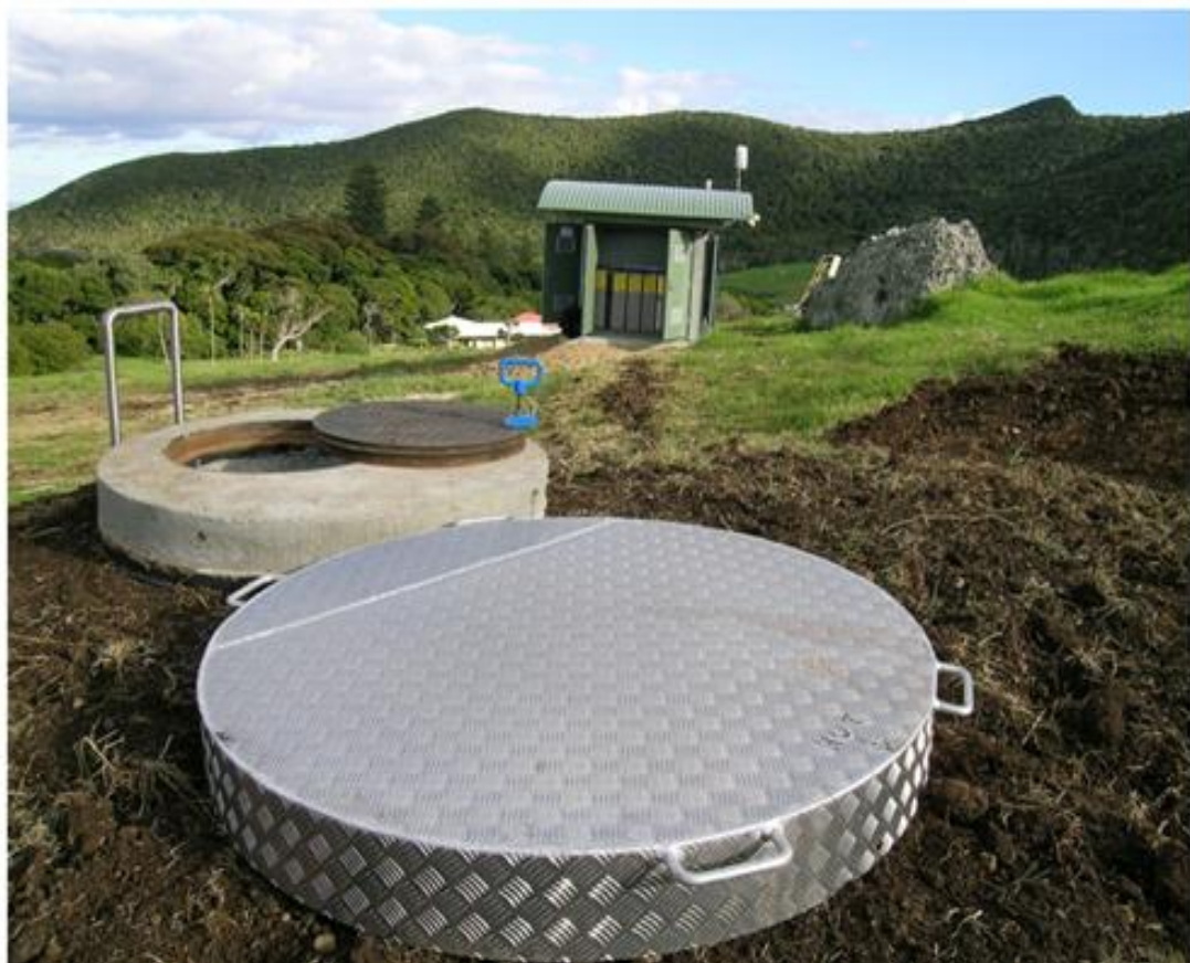
Figure 3. The seismic monitoring station at Lord Howe Island. In the foreground are the top of the seismic vault and vault cover with the hut containing the electronic processing equipment and battery bank in the background.
