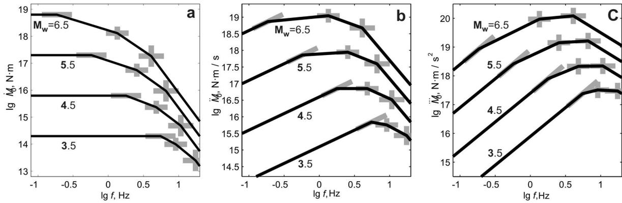
**Figure 3.** Families of average source spectra  $\dot{M}_0(f)$  (a),  $\ddot{M}_0(f)$  (b) and  $\ddot{M}_0(f)$  (c) for earthquakes of Kamchatka (lines), and  $\pm 1\sigma$  ranges of scatter of individual spectra (grey bars): along ordinate - for their level, and along abscissa - for corner frequency position.
