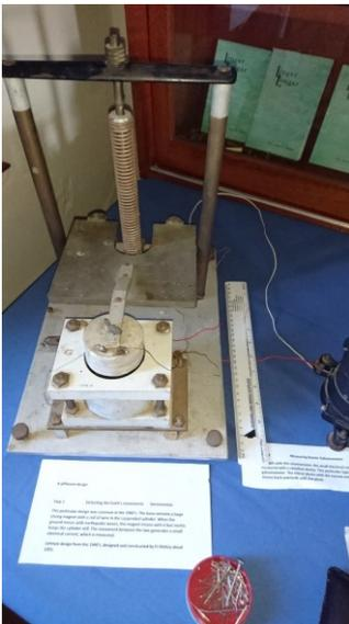
Figure 3. Wilson Lamerson seismometer - University of Qld model - also built by Fr. Joe McKey
