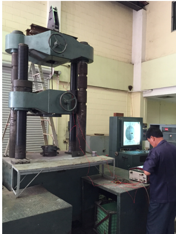
Figure 2 Test setup of CFD (located on top of universal testing machine) over reversed cyclic displacement
