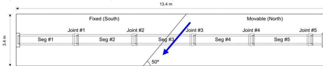
**Figure 4.** Layout of the segmented concrete pipeline crossing fault (Kim Junhee, 2010)
