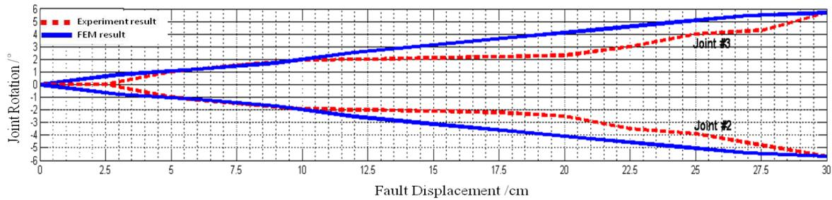
**Figure 6.** Effect of fault displacement on joint rotation
