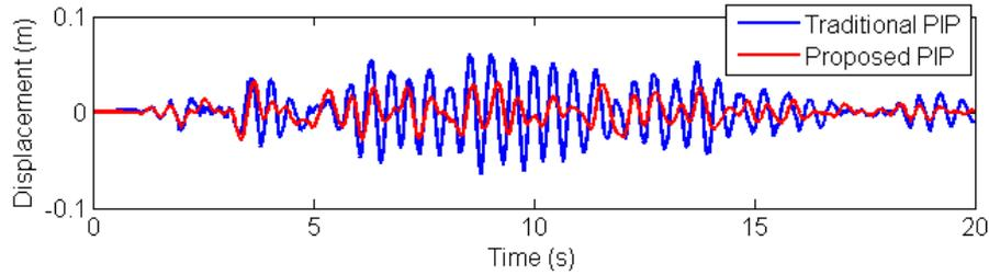
Figure 10. Transverse displacements of the inner pipe at the middle of the free span when the proposed and traditional pipe-in-pipe systems are subjected to the transverse earthquake loading
