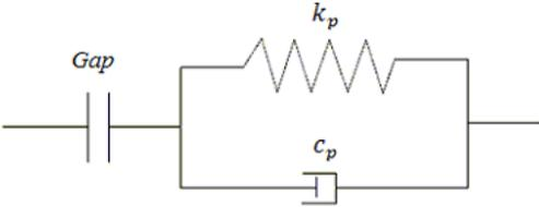
Figure 6. A typical impact element
