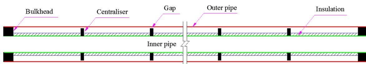
Figure 1. A typical pipe-in-pipe system (not to scale)
