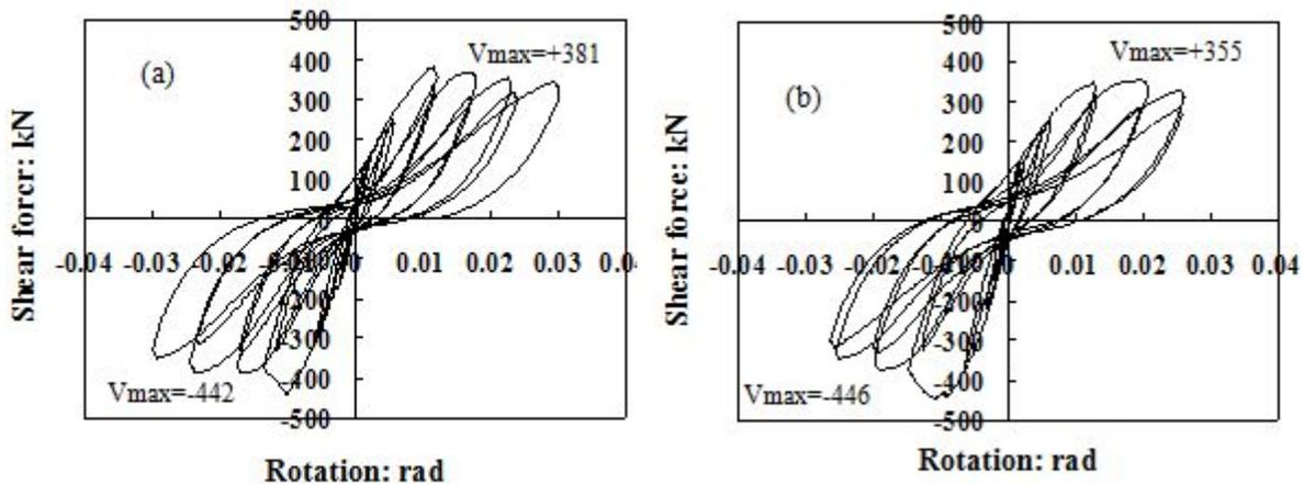
Figure 6. Load-rotation curves: (a) DCB10; (b) DCB11
