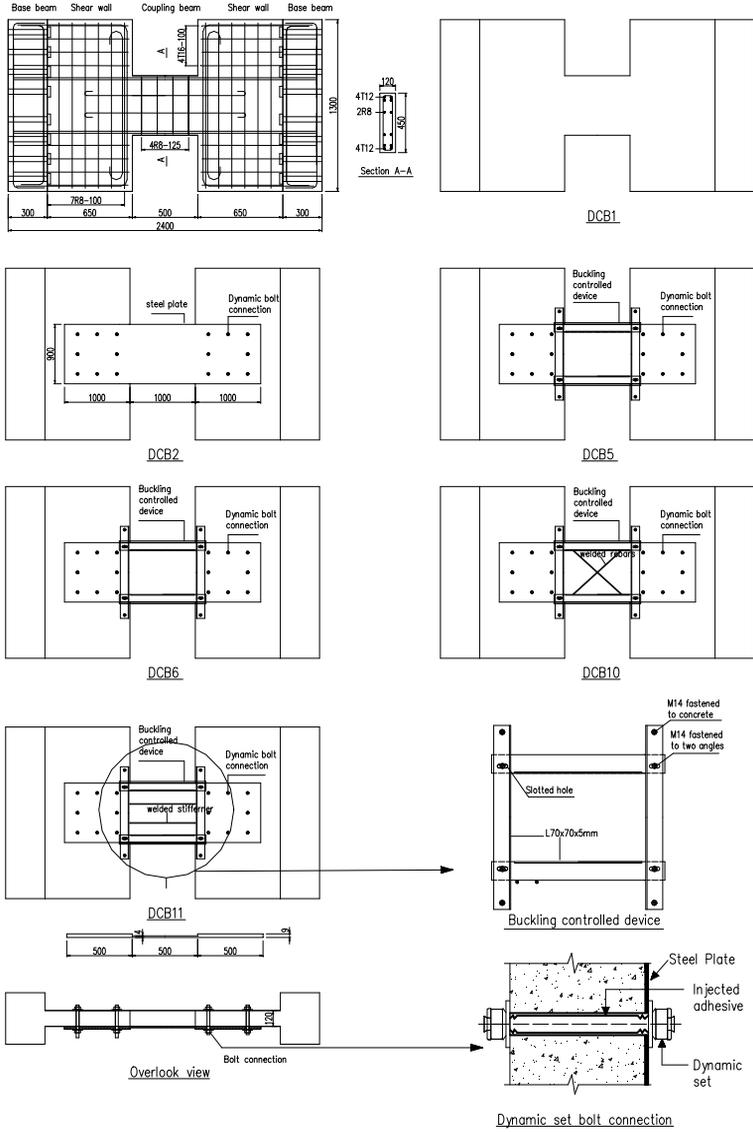
**Figure 1. Details of test specimens**
