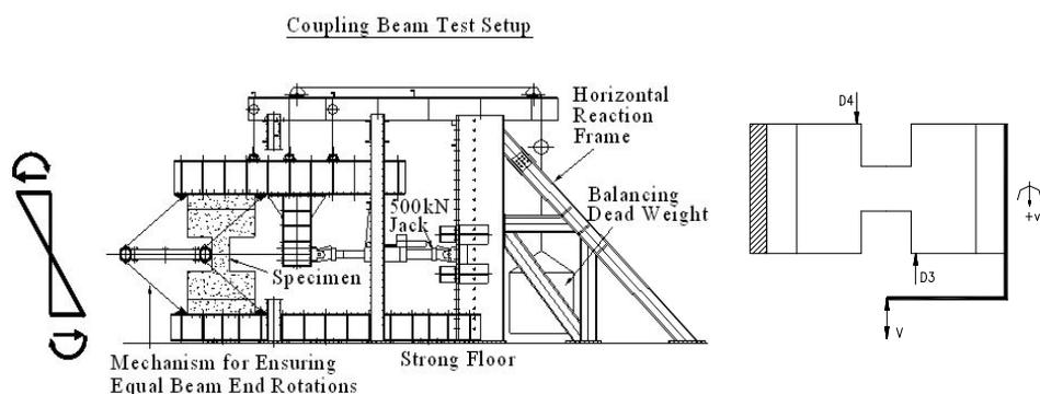
**Figure 2. Test setup**
