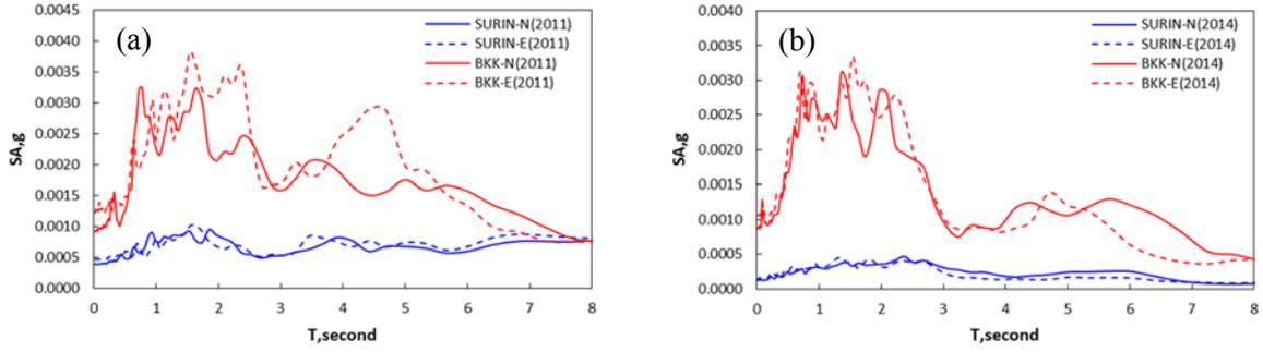
Figure 1. Spectral Acceleration at Bangkok (soft soil) and Surin station (stiff soil) (a) 2011 event, (b) 2014 event.
