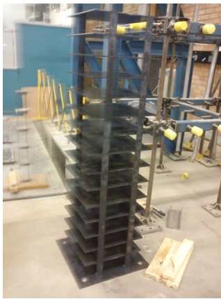
Fig.2. Completed structural model
