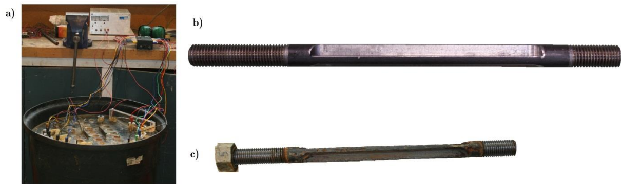
Fig. 3: a) Corrosion test setup of dissipater, b) a non-corroded dissipater, and c) a corroded dissipater
