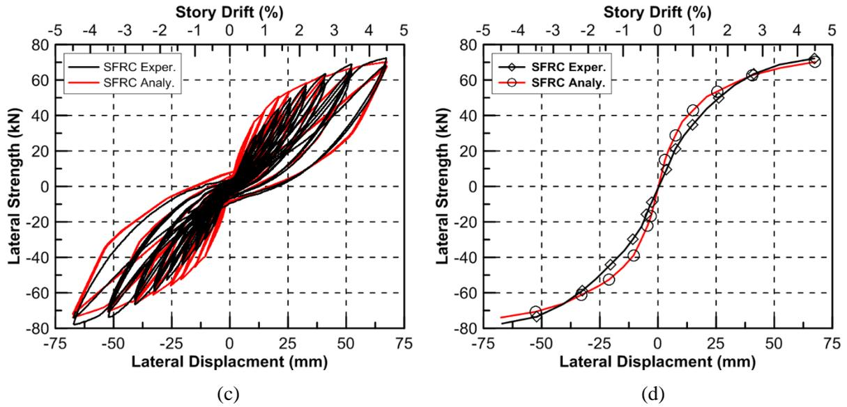
Figure 6. (a, c) Hysteresis comparison of RC and SFRC frames, (b, d) Backbone comparison of RC and SFRC frames
