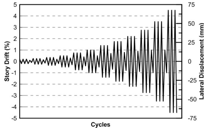
Figure 5. Cyclic Displacement profile applied on study frame
