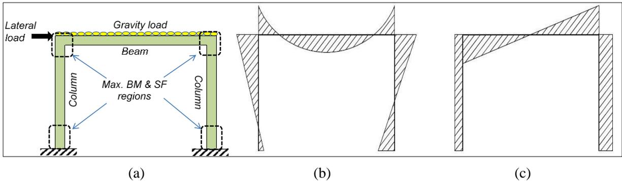
Figure 1. (a) Study frame under constant gravity loading and lateral loads showing plastic hinges zone, (b) BM diagram for given loading, (c) SF diagram for given loading.
