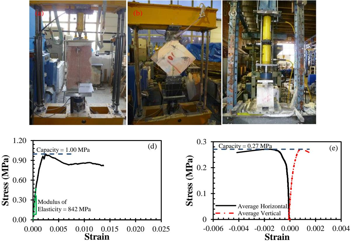
**Fig. 2 – Material test setups and test results : (a) Compression test setup , (b) Diagonal tension test setup, (c) Triplet test setup, (d) Compressive stress-strain curve and (e) Diagonal tension stress-strain curves**
