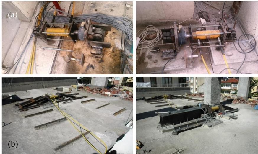
**Fig. 5 – Photos of hydraulic actuators at each story : (a) First story and (b) Roof**
