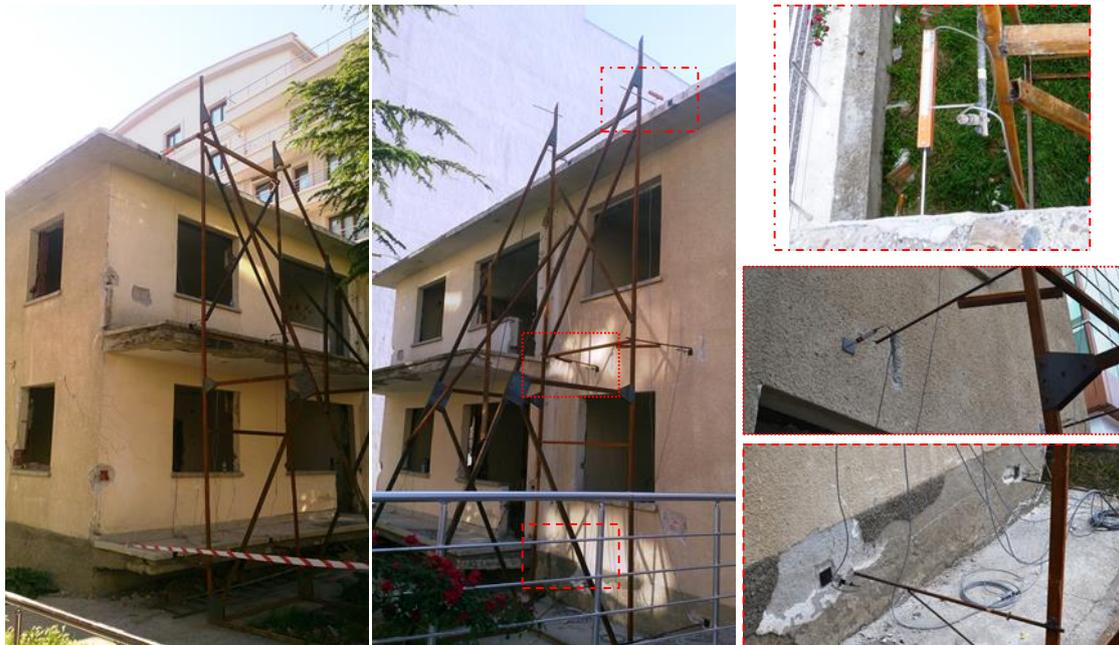
**Fig. 6 – Photos of LVDT's installed at each story level**
