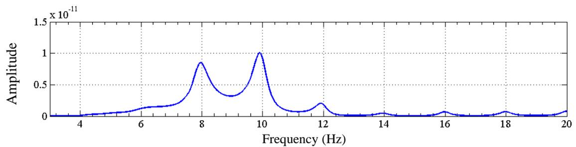
**Fig. 4 – FFT of transfer function for recorded accelerations**
