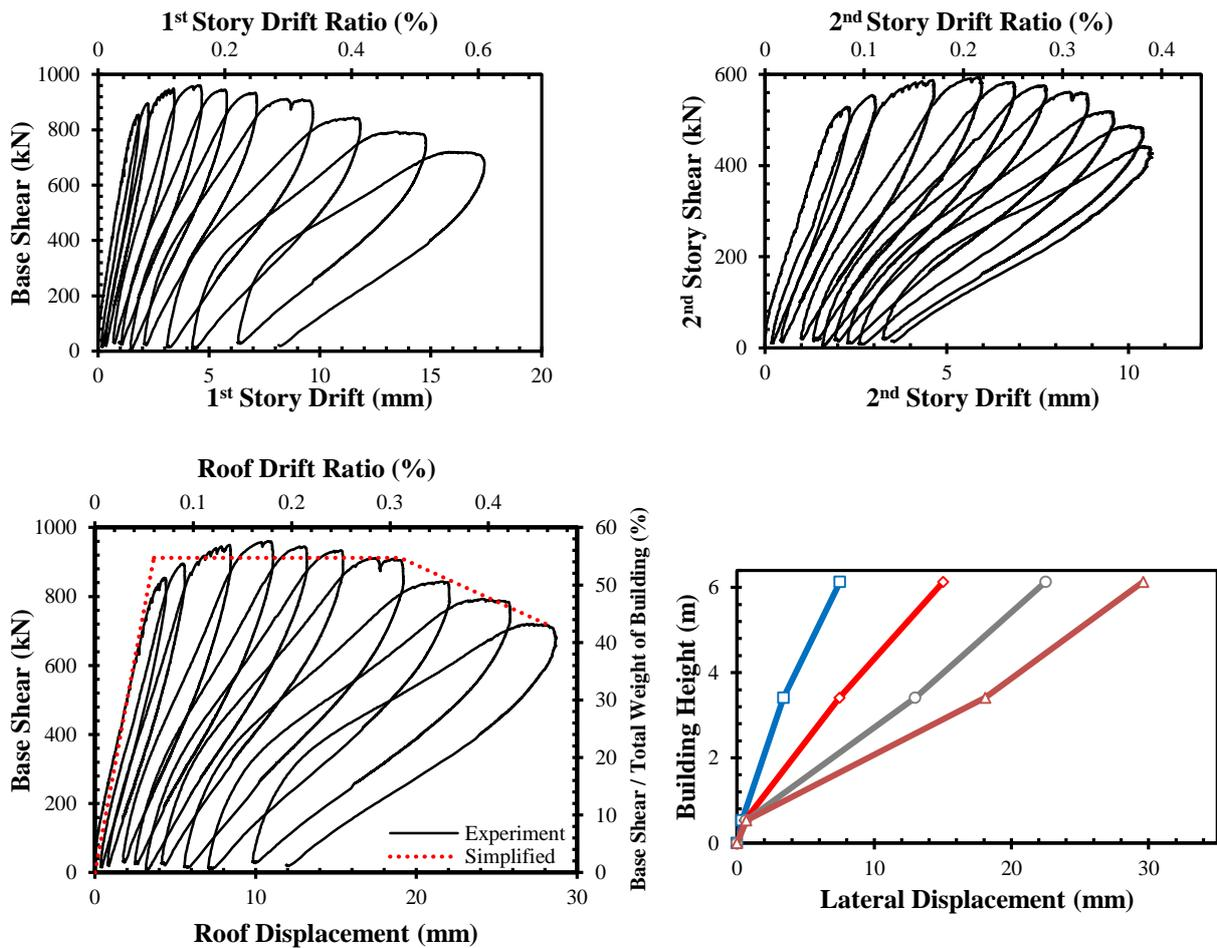
Fig. 8 – Recorded load – deformation responses
