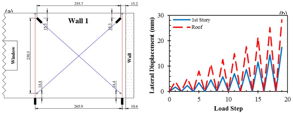
Fig. 7 – (a) The installed LVDT's for a representative wall and (b) Control displacements applied to each story \*All units are in cm.
