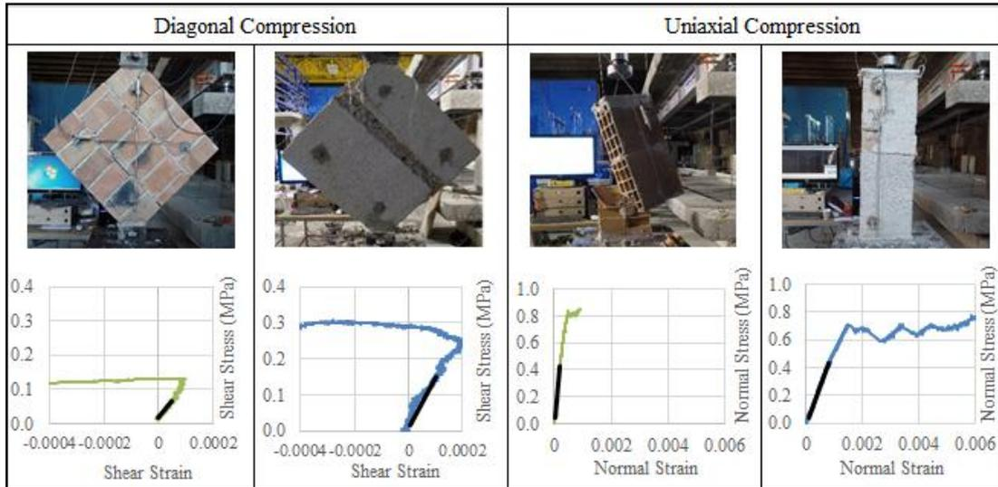
**Fig 2. Prism failure modes and stress-strain curves**
