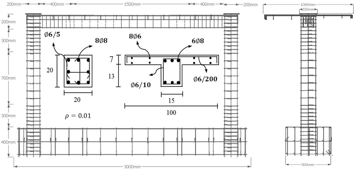
Fig 3. Reinforcement details of the test frame
