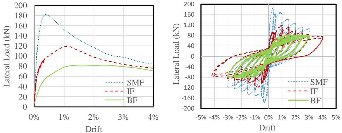
**Fig 8 Backbone curves and hysteretic responses of tested frames**
