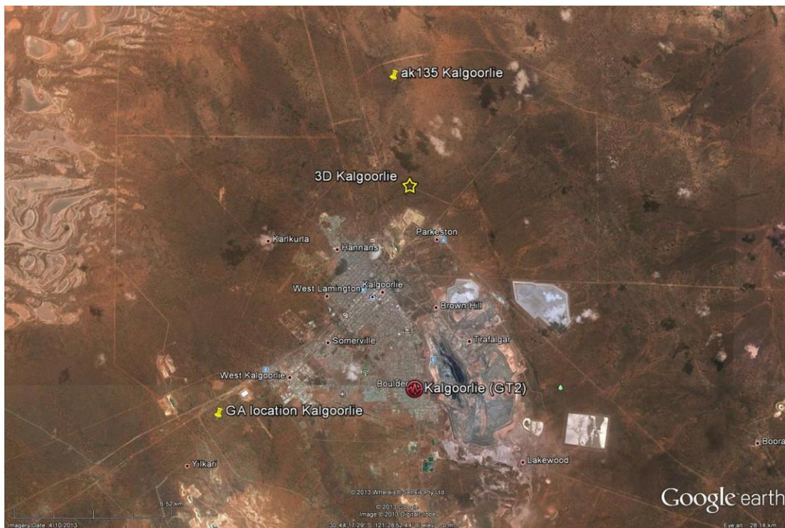
Figure 4. Kalgoorlie: This mb5.0 earthquake was well located using a local mine monitoring network. Location errors are  $d(\text{ak135})=12.6$  km,  $d(3\text{D})=8.3$  km and  $d(\text{GA})=8.3$  km. Using only P and S phases on 7 stations < 6 degrees distant this improves to  $d(\text{ak135})=9.6$  km and  $d(3\text{D})=4.5$  km.
