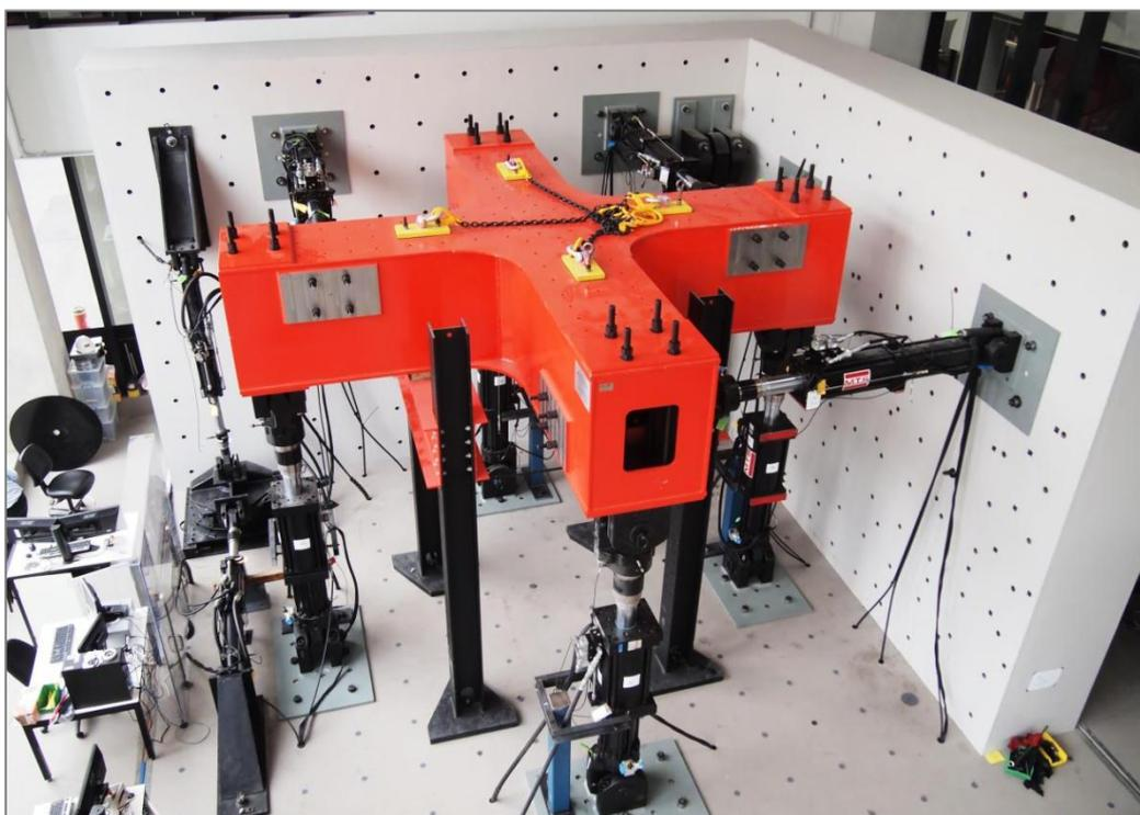
Figure 2. MAST System in Smart Structures Laboratory at Swinburne
