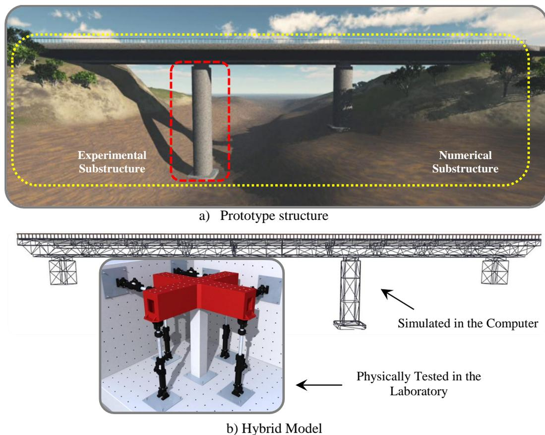
Figure 1. Hybrid simulation technique
