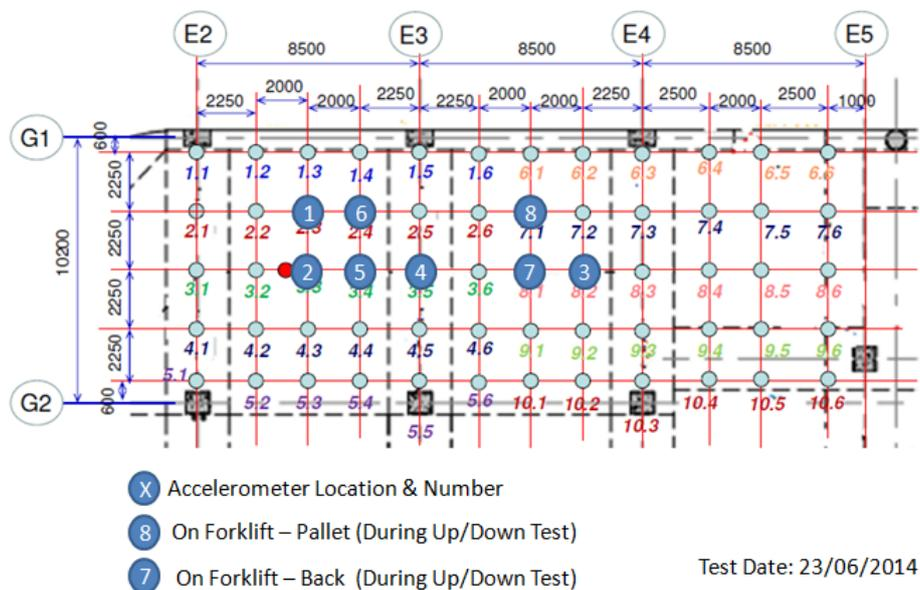
Figure 1: Forklift up-down and back-forth test sensor locations
