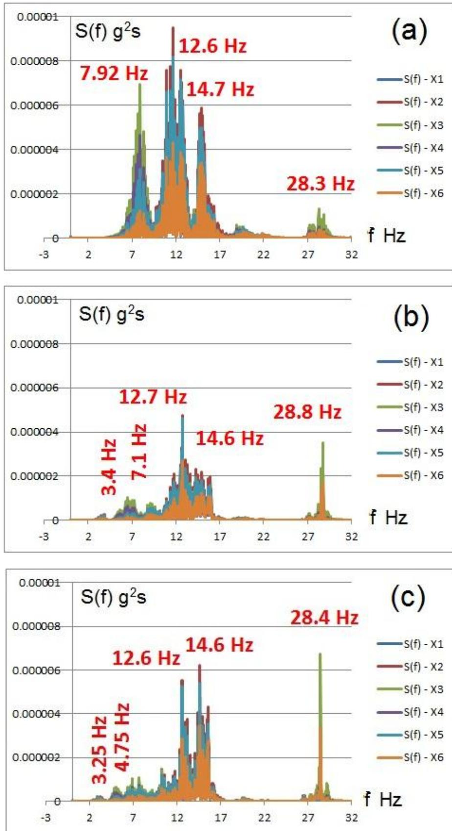
Figure 5: Acceleration response spectra at all six floor grid points for up/down mast motion
