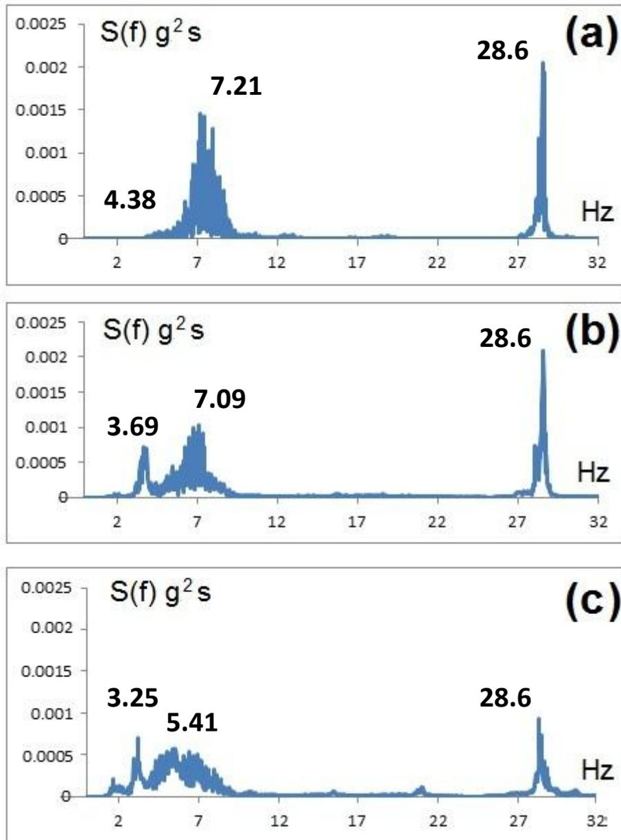
**Figure 4: Acceleration Response Spectra at central payload position
