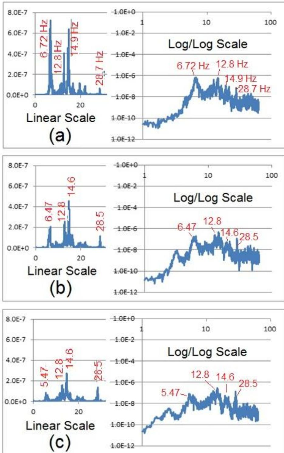
**Figure 7: Acceleration response spectrum at floor location X5 for back-forth forklift motion**
