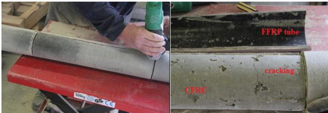
Figure 3. FFRP-CFRC column after removed the outer tube
