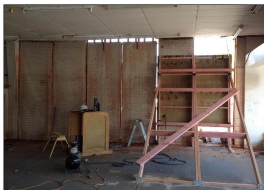
(c) Test reaction frame after testing Has-W1 to complete collapse and prior to testing Has-W2
