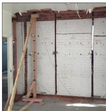
(a) Instrumentation framing at Auc-W3 after Auc-W1 and Auc-W2 have been tested and cracked
