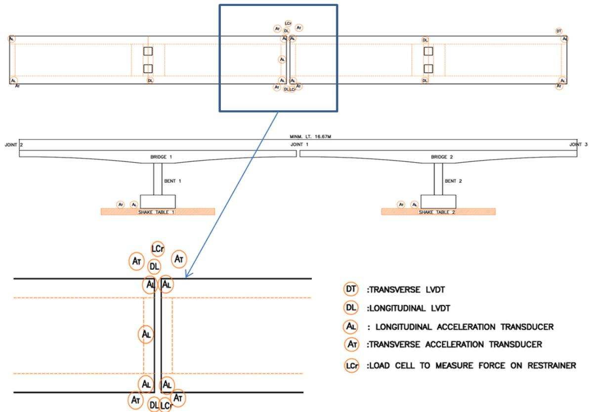
Figure 2. Instrumentation details of the bridges
