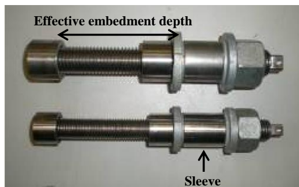
Figure 2. Headed anchor blind bolt (HABB)
