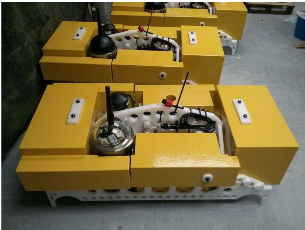
Figure 1. Photo of OBS recorders prior to initial deployments, note that ballasts have not yet been attached.
