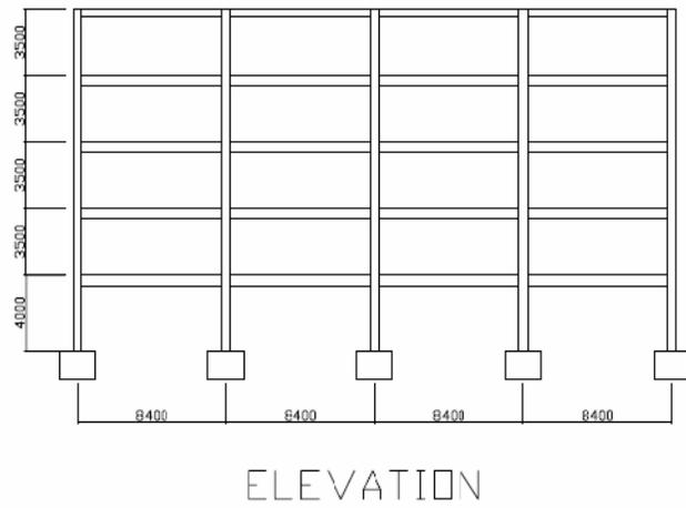
**Figure 3 Building elevation**
