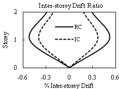
Figure 9 – Inter-storey drift ratio (400 kN/m, 0.25 metre clearance)
