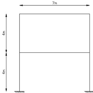
Figure 1 – Reference structure with fixed floor slab (RC)
