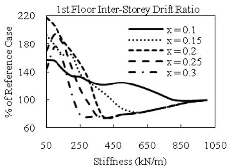
Figure 5 – 1<sup>st</sup> floor inter-storey drift ratio for varying stiffness and clearance distance
