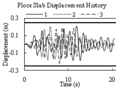
Figure 11 – Floor slab displacement time history (400 kN/m, 0.25 metre clearance)
