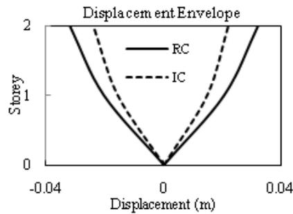
Figure 8 – Displacement envelope (400 kN/m, 0.25 metre clearance)
