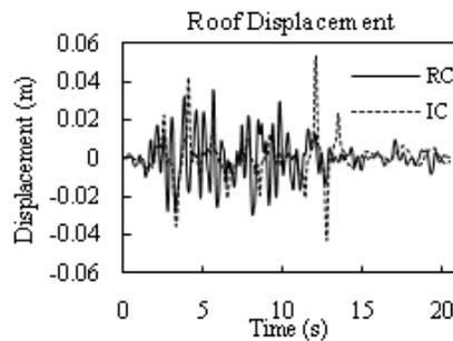
Figure 10 – Roof displacement time history (200 kN/m, 0.15 metre clearance)
