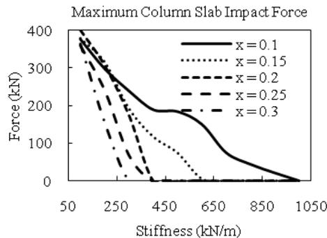
Figure 20 – Column – slab impact force
