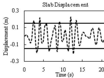
Figure 12 – Floor slab displacement time history (200 kN/m, 0.15 metre clearance)
