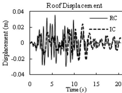
Figure 7 – Roof displacement time history. (400 kN/m, 0.25 metre clearance)
