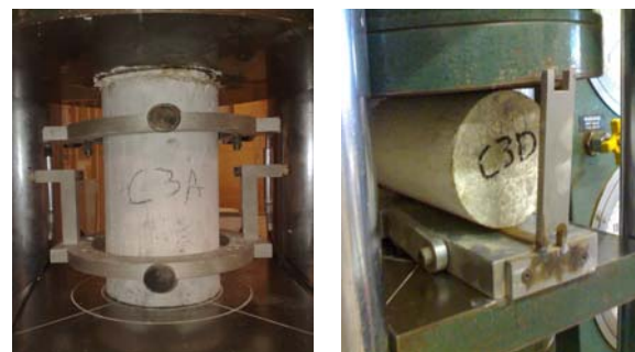
(a) MOE testing (b) STS testing
