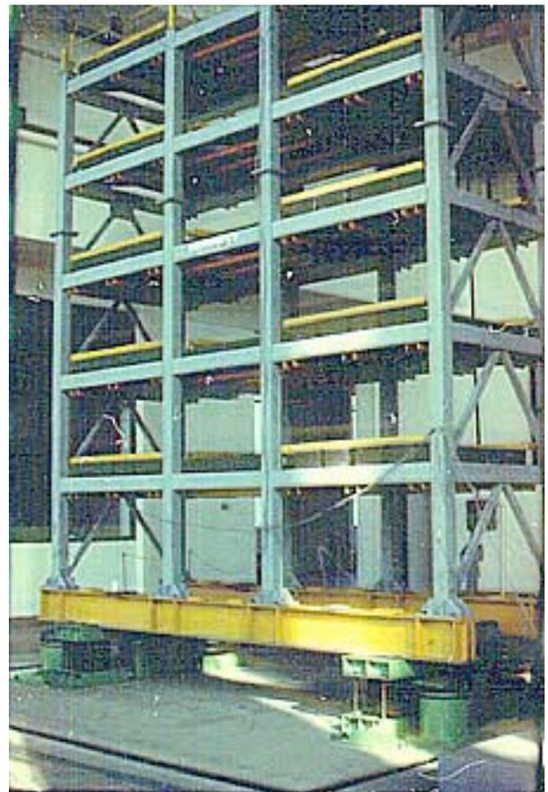
**Figure 1** Shaking table test of a 5 storey steel frame model Isolated by GERB Vibration Isolation Elements at IZIIS Macedonia (joint program with GERB Germany).
