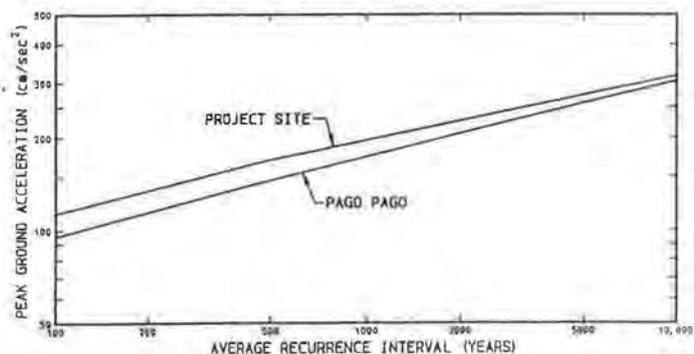
Figure 2 Peak Ground Acceleration Versus Average Recurrence Interval
