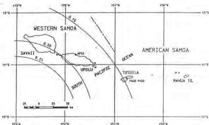
Figure 3 Acceleration Coefficient Contours for Samoa (500 year average recurrence interval)
