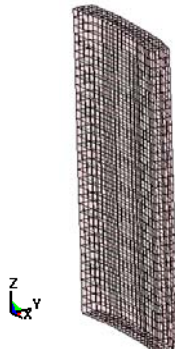
Figure 12. Deformed shape when maximum deflection reaches ( t=66 msec)
