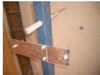
Figure 5. Deflection measurement device
