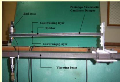
Viscoelastic Damper, Attached to a Beam
