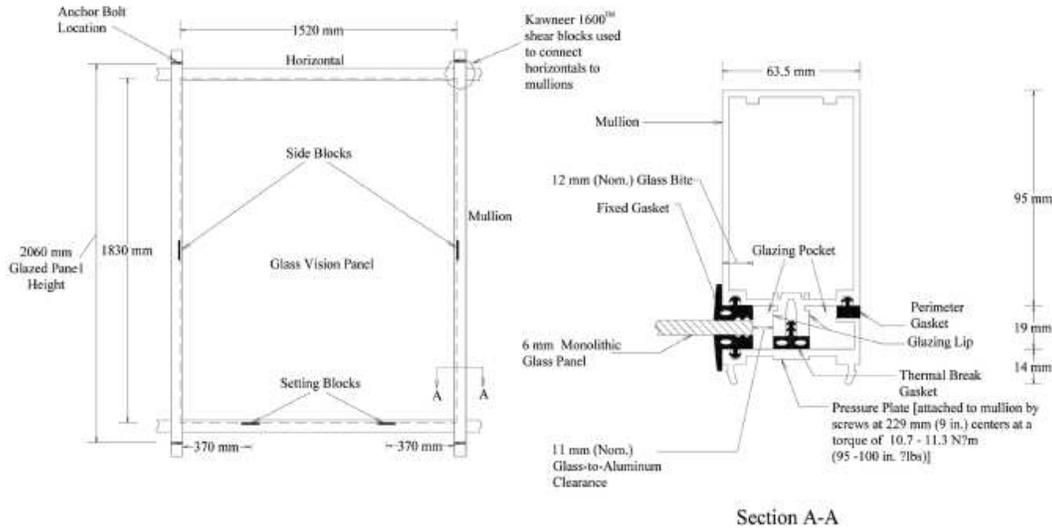
Figure 5 General glazing details for curtain wall mock-up test (Memari et al. 2007)
