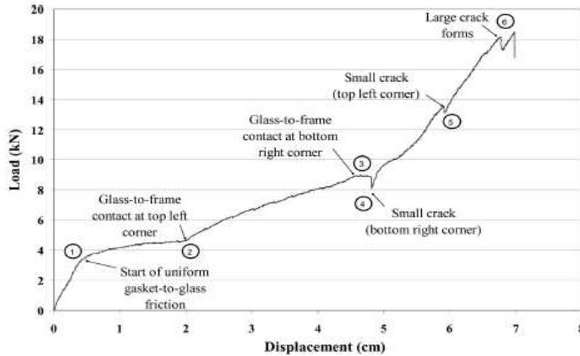
Figure 7 Load-displacement relationship during static (0.01 cm/sec) racking test (Memari et al. 2007)
