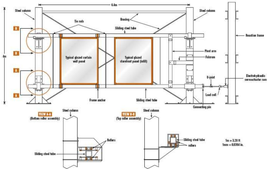
Figure 2 Dynamic racking test (Saflex Solutia Architectural Glazing 2007)
