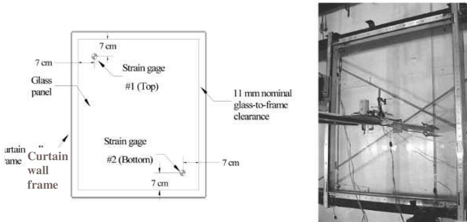
Figure 6 Strain gage locations on architectural glass curtain wall mock-up (Memari et al. 2007)
