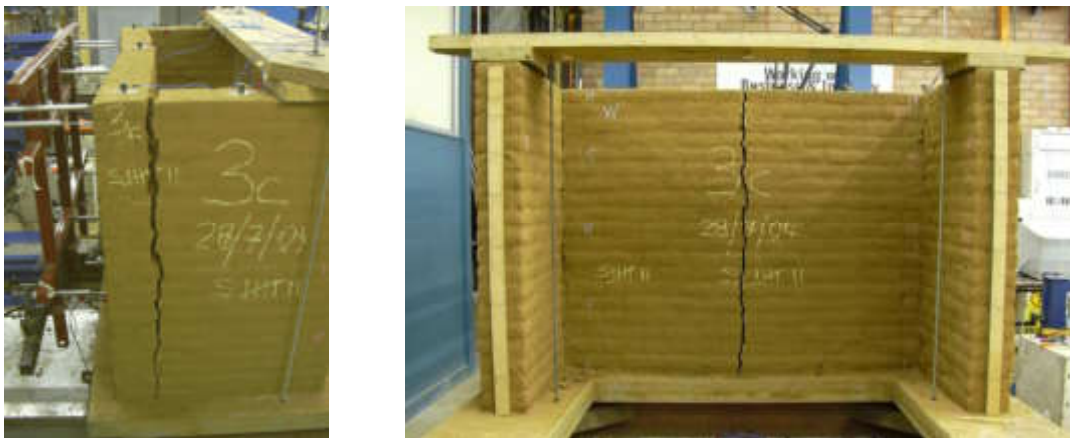
Figure 6a&b. Vertical corner cracking and mid-span vertical cracking of Specimen 3C (with horizontal mesh reinforcement) after shake table testing (Dowling, et al., 2004)
