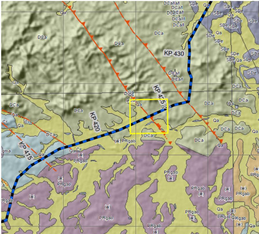
Figure 4 – Geologic map of the southern end of the Queenslandler Fault. The yellow box defines the detailed map areas of Figure 5.
