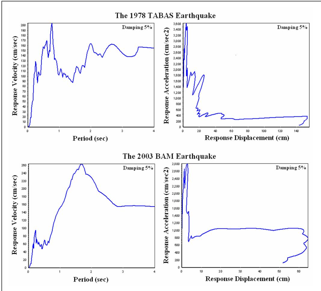
Figure 5: Response velocity spectra and acceleration-displacement spectrum due to fault normal component of main shock of the 1978 Tabas and 2003 Bam earthquakes.
