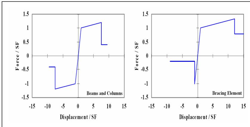
Figure 4: Assumed non-linear behavior for the structural hinges
