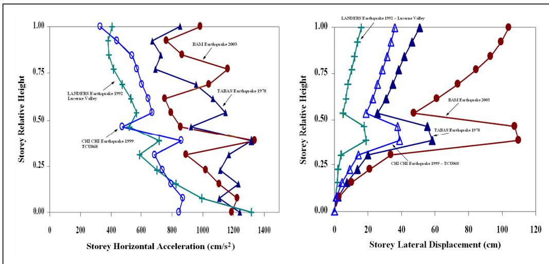
Figure 6: Total acceleration and lateral displacement results form the dynamic response of thirteen storey building to the near field records as notified in Table 2.
