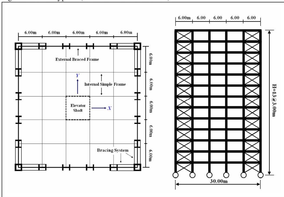
Figure 3: Structural system of the example 13-storey building
