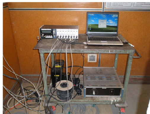
(b) Data acquisition box and laptop for operation and collection of data
