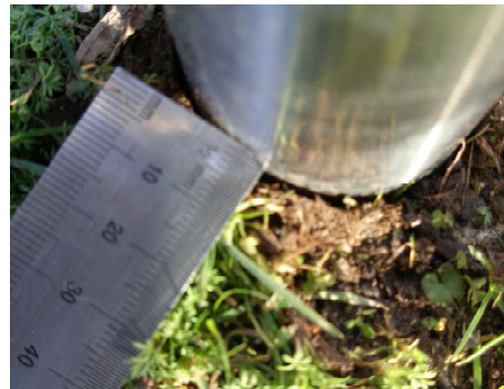
Figure 4 Pile-soil gap at 1.5 mm
