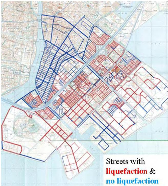
Fig. 24 Distribution of liquefaction in Urayasu City
