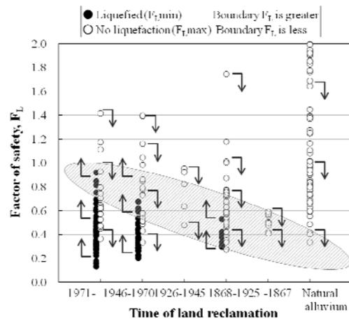
Fig. 33 Revised insights on ageing effect on the border value of  $F_L$  between liquefied and unliquefied sites
