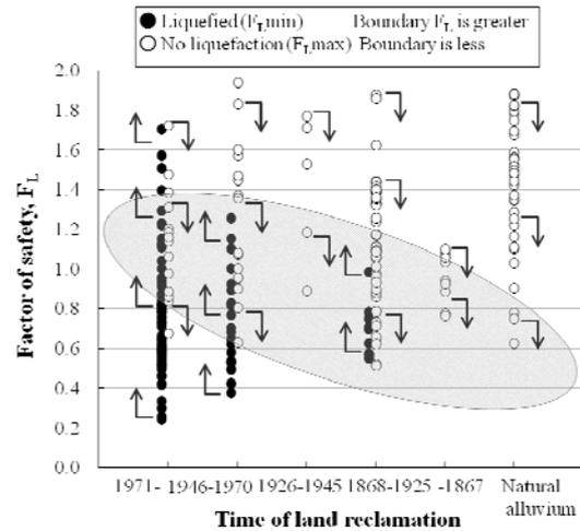
Fig. 32 Possible ageing effect on the border value of  $F_L$  between liquefied and unliquefied sites
