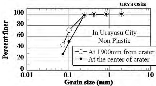
Fig. 17 Grain size distribution of ejected sand
