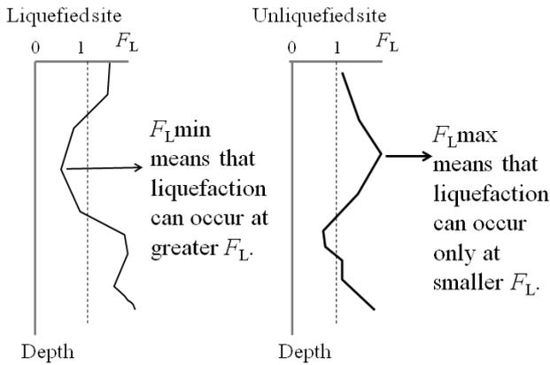
The boundary between  $F_L$  for liquefaction and  $F_L$  for no liquefaction lies between  $F_{Lmin}$  and  $F_{Lmax}$ .
