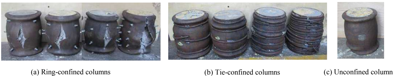
Fig 7 Failure modes of tested columns
