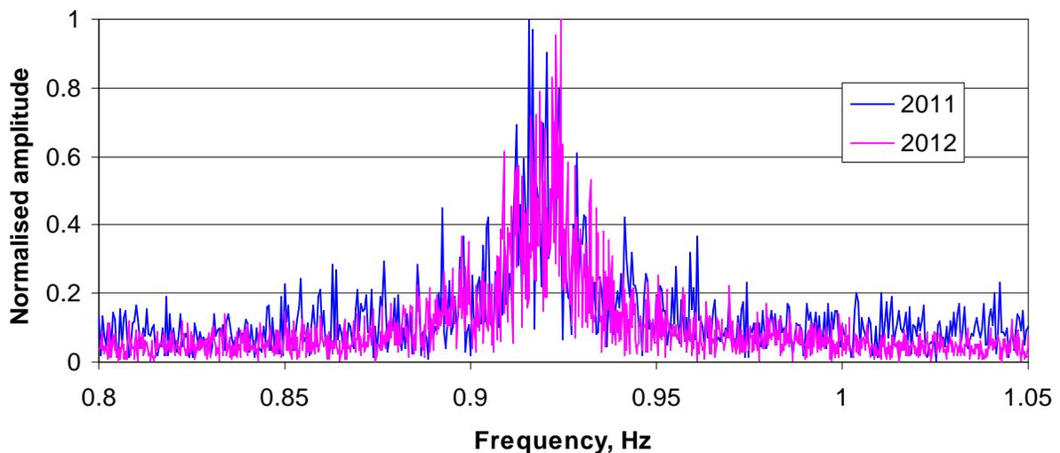
**Figure 5 - Normalised spectrum of Sydney Harbour Bridge vertical acceleration showing the fundamental natural period ( $\approx 0.92$ Hz), measured on the 28th October 2011, and the 2nd July 2012. Higher order modes show similar frequency shifting.**
