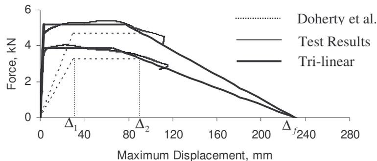
Figure 5: Obtained force-displacement curves, tri-linear representation
