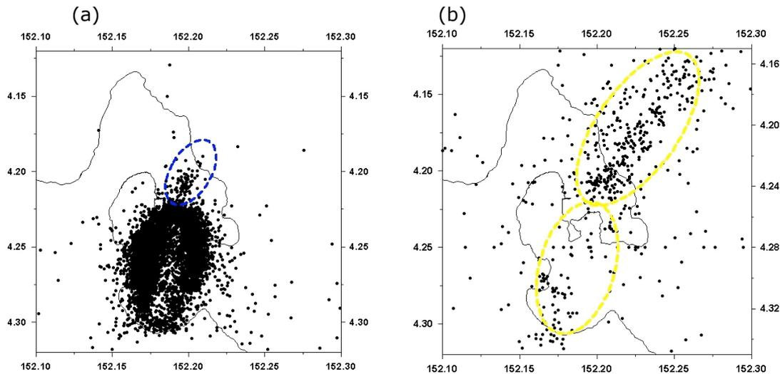
Fig. 1: Seismicity of Rabaul Caldera, (a) before the 1994 eruption, and (b) after the eruption. The pre-eruption northeast earthquakes are marked by the dashed ellipse in (a).
