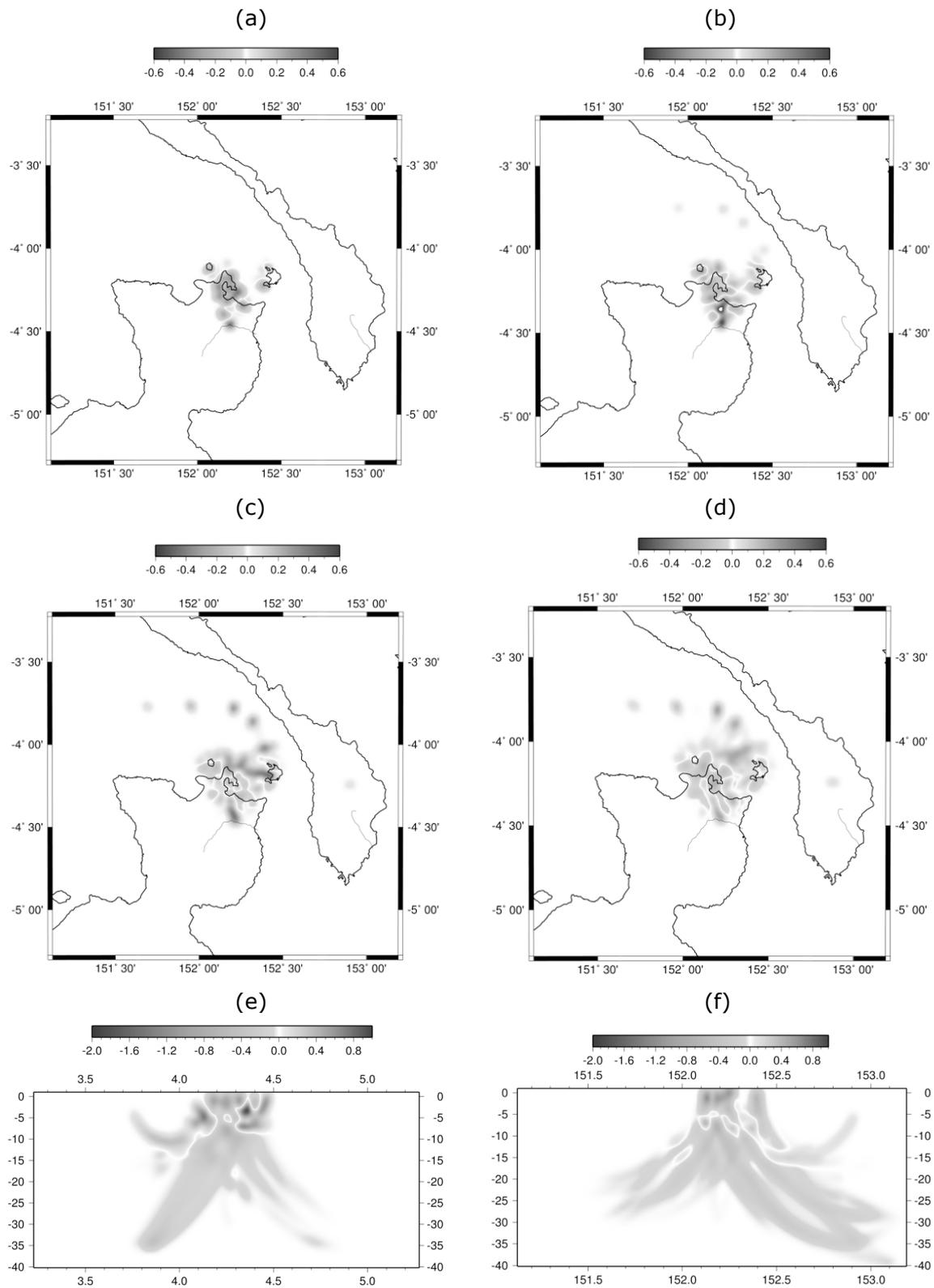
Fig. 3: Preliminary tomographic results showing relative velocity perturbations for 1, 3, 6 and 8 km depth slices (a-d), and north-south and east-west cross-sections (e-f). The north-south cross-section is sliced through longitude 152.18°E and the east-west cross-section through 4.24°S, both of them passing through the center of the caldera.
