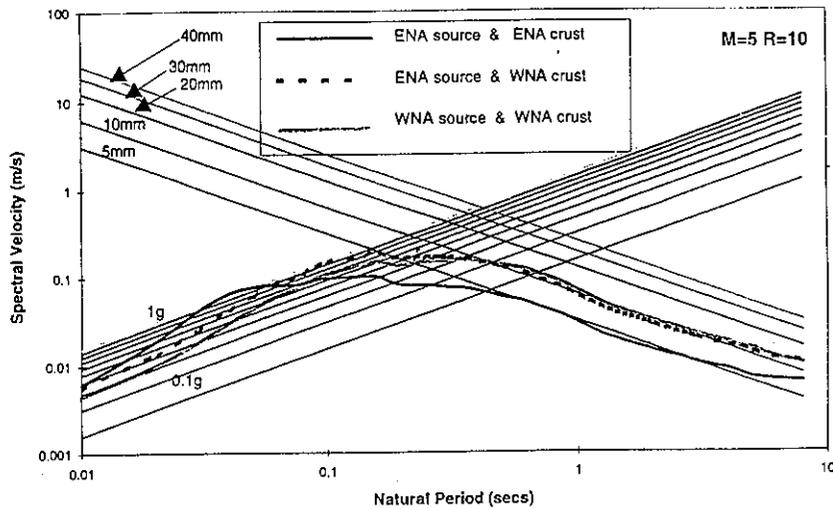
Figure 3 Response Spectra associated with ENA & WNA Crust Models
