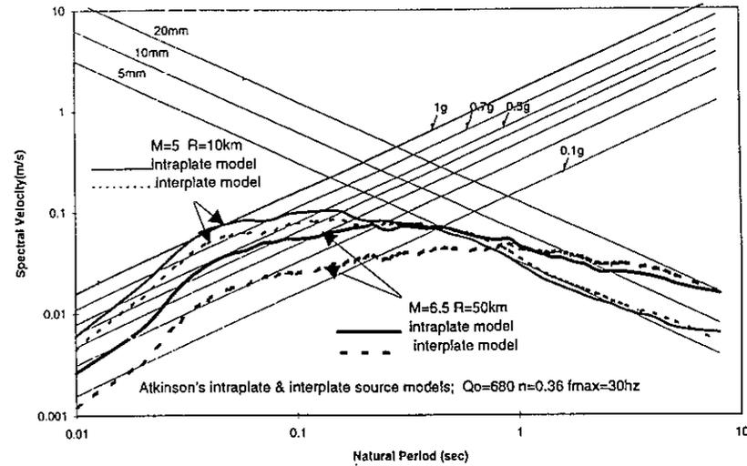
Figure 2 Response Spectra associated with ENA & WNA Source Models
