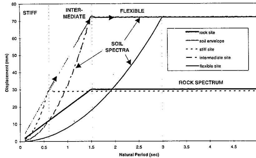
Figure 4 Displacement Spectra of Rock and Soil Sites
