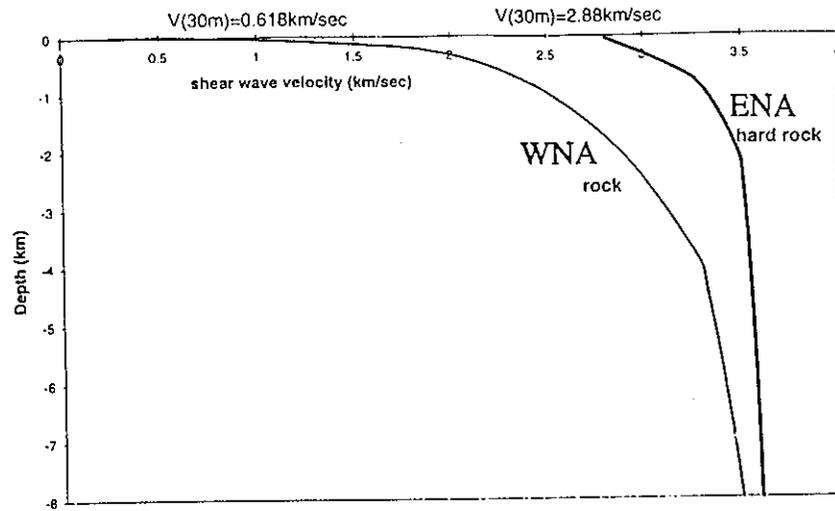
Figure 1 Shear Wave Velocity Gradients of the Generic Crust Models
